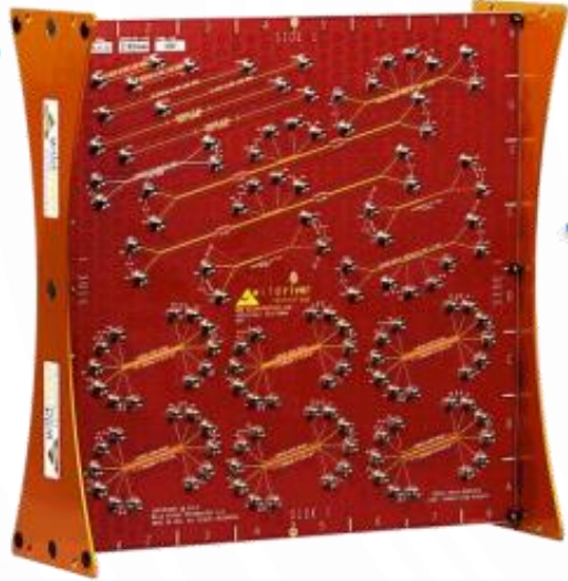
Crosstalk Noise Test vehicle, calculated RX noise as Integrated Crosstalk Noise (ICN)
